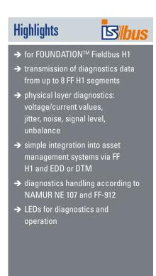
The Diagnosis Communication Module (DCM) transmits advanced physical layer diagnostics data, measured by the ISbus Fieldbus Power Supplies, to a host and/or asset management system via FF H1 communication.
