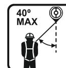
Permissible inclination of work line from the vertical line
