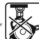
Do not attach the device to a structural anchor point (anchor point) using handle for device transportation
