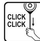
Before each use check function of the locking gear.
